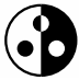
Figure 28.11 SATURATION control in a decoder alters chroma gain. The comparable control in processing equipment is CHROMA GAIN.
