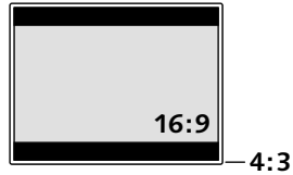
Figure 1.4 Letterbox format fits widescreen material – here, 16:9 – to the width of a 4:3 display.
