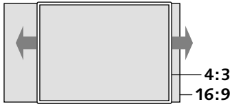
Figure 1.3 Pan-and-scan crops the width of widescreen material – here, 16:9 – for a 4:3 aspect ratio display.
