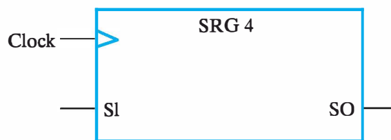
□ FIGURE 7-9 4-Bit Shift Register
