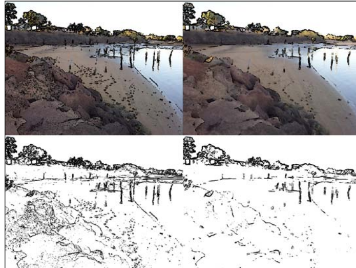
Left: Sobel filter, Right: 3x3 Blur + Sobel filter
