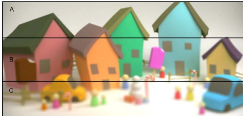
Uniform box blur using varying kernel sizes: 3x3 (A), 5x5 (B), and 9x9 (C)
