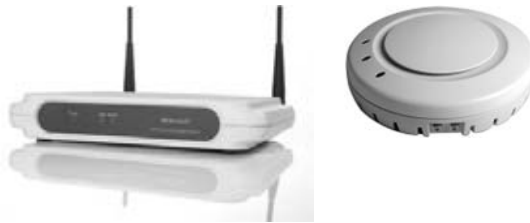
FIGURE 10.2 WIDS/WIPS hardware sensors
