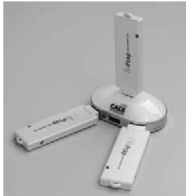
FIGURE 7.20 AirPcap provides multichannel monitoring and roaming analysis.
