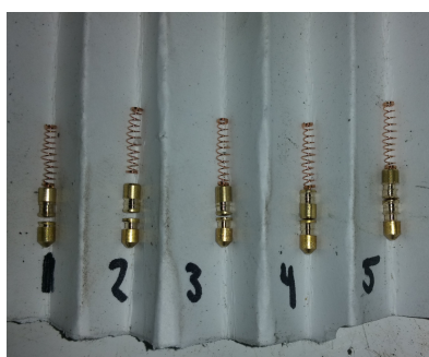
Fig 6) Aim to cut serrations or spool shapes into the pin.
