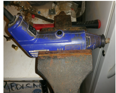
Fig 1) A dremel/high speed rotary tool.
